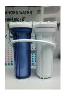
On the left hand side is fiber filter, and on the right hand side can choose installation of KDF filter, Ion exchange resin filter or Anti-bacteria carbon filter. It can be added one more white case to become a 3 stage filter system. They are used to remove the contamination in water. Please change the fiber filter when it changed to brown in color completely. All kind of pre-filter water pressure cannot exceed PSI 20.
